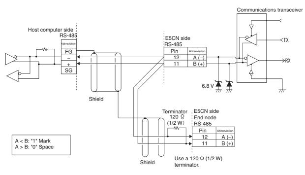
Specify both ends of the transmission path including the host computer as the end node (that is, connect terminators to both ends). Use a terminating resistance of at least 54  $\Omega$ .
