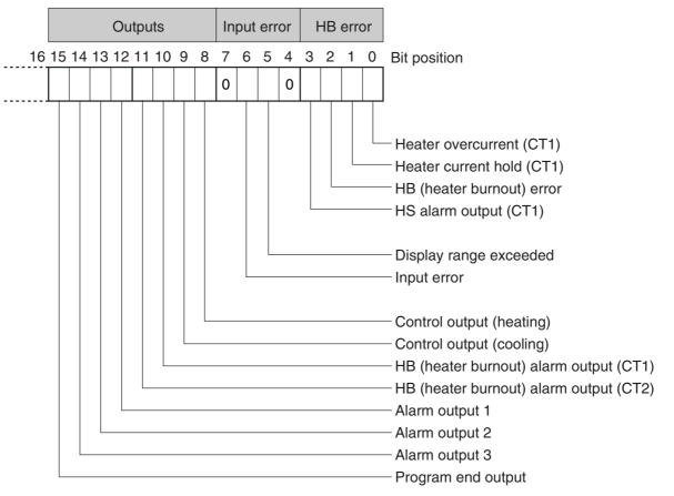
The figure below shows the structure of the status data.
