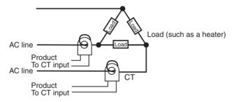
Star connecting lines: Refer to the following diagram for CT installation positions.
