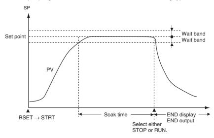
• The program will start when the "program start" parameter is changed from RSET to STRT. END will be displayed on the No. 2 display and the output assigned as the program end output will turn ON after the time set in the "soak time" parameter has expired in the wait band. The "program pattern" parameter can be used to select moving to STOP mode or continuing operation in RUN mode after the program ends.
