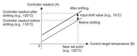
Figure 2 Illustration of 1-Point Shift
