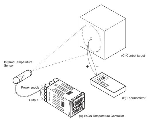
Figure 1 Offset Configuration for an Infrared Temperature Sensor
