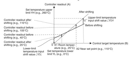
Figure 3 Illustration of 2-Point Shift
