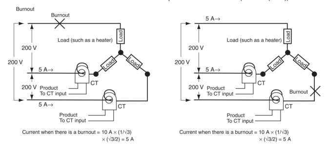
The heater burnout detection current for this connecting line is 5.4 A (= (5.8 + 5) / 2).
