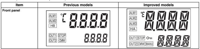
Basically, the Controllers are upwardly compatible. The terminal arrangement, terminal sizes, and depth for panel mounting have not been changed. Changes are listed in the following tables. For details, refer to the pages given for specific items in the index.
