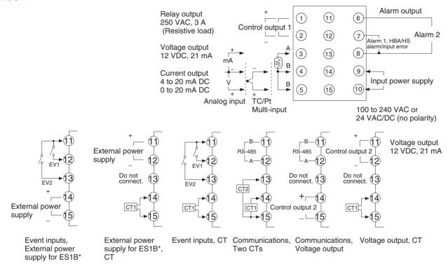
\*The external power supply for ES1B cannot be used on the E5CN-C (Current Output Model).
