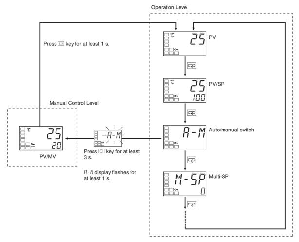
• If an event input is set to "MANU" (auto/manual), the "auto/manual switch" parameter will not be displayed. Use the event input to switch between automatic and manual modes.
