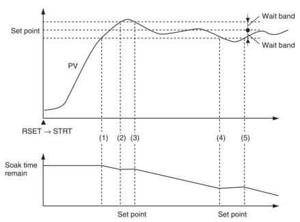
The wait band is the fixed band within which the process value is stable in respect to the set point. The soak time is measured within the wait band. The timer that measures the soak time operates only when the process value is within the wait band around the set point (i.e.,  $SP \pm$  wait band). In the following diagram, the timer will be stopped between the start and (1), (2) and (3), and (4) and (5) and will measure the time only between (1) and (2), (3) and (4), and (5) and the end.
