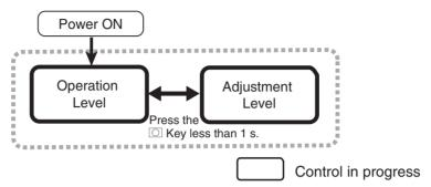
To move to the adjustment level from the operation level, press the  $\ igtimes$  key once.
