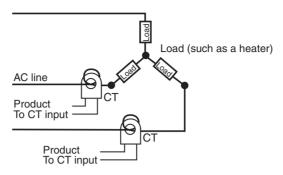
3. V connecting lines: Refer to the following diagram for CT installation positions.
