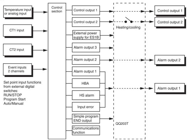
**Note** Functions can be assigned individually for each output by changing the set values for the control output 1 assignment, the control output 2 assignment, the alarm 1 assignment, and the alarm 2 assignment in the advanced function setting level.
