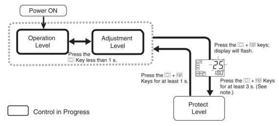
To move from the operation level to the protect level, press  $\bigcirc$  and  $\boxdot$  keys for three seconds (see note) or more.
