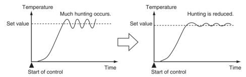
When the temperature (PV) falls short of the set point for the PID constants when using AT or ST in normal mode, executing AT or ST in RT mode tends to improve performance.
