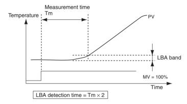
3. Set the "LBA detection time" parameter to two times the measured time.
