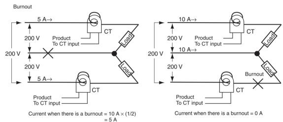
The heater burnout current when there is a burnout at the common is as follows:
