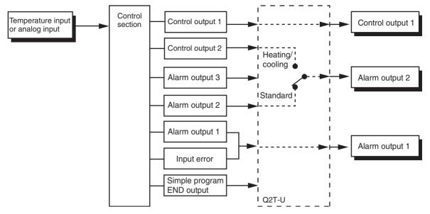
**Note** Functions can be assigned individually for each output by changing the set values for the control output 1 assignment, the alarm 1 assignment, and the alarm 2 assignment in the advanced function setting level.
