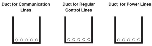
If the wires must be placed in the same duct, separate them via an earthed/grounded divider.
