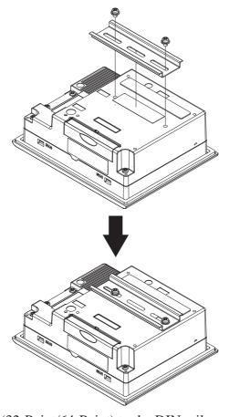
2) Attach the Unit (32-Point/64-Point) to the DIN rail.
