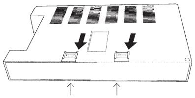
There are two retaining tabs on this side of the Unit.
