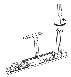
5. Raise the retaining bracket and insert the ISA board into the ISA connector. The ISA board must be facing the right direction. Make sure that the connectors are aligned and press the board firmly into place.
