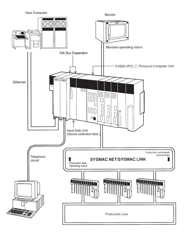
In this example an Ethernet board and modem board have been installed in the 2 ISA Bus Expanders.
