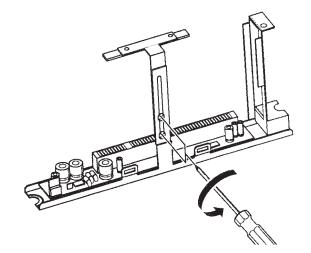
4. Remove the board retaining screw. The following diagram shows the location of this screw.
