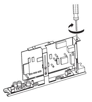
7. Check that the retaining bracket fits snugly against the ISA board and tighten the bracket screws. Torque the screws to 0.54 N-m.
