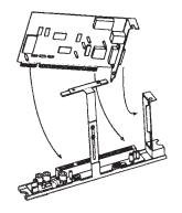
6. Tighten the board retaining screw. Tighten the screw to 0.54 N-m.
