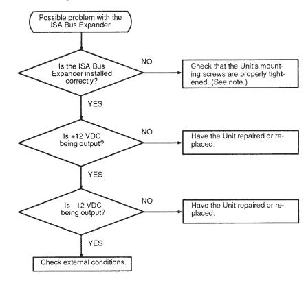
**Note** Refer to *3-3 Installing the ISA Bus Expander* for details on mounting the ISA Bus Expander to the CPU Backplane.
