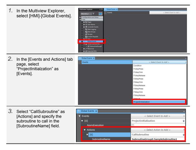
• Creating the Subroutine That Runs Upon Activation/Deactivation of an Alarm Event In the NS series, a macro can be run upon activation or deactivation of an alarm. In the NA series, it can also be run even at the timing of confirming an alarm.
